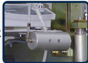
Pneumatic valve slurry feed Analogic control
